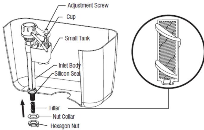
1. Unscrew Hexagon nut and Nut collar from the Fill valve, insert Fill valve with Silicon seal into the inlet hole of Water tank and make sure Fill valve is in the right position, then screw Nut collar and Hexagon nut in turn to Fill valve tightly. Then connect Refilling tube with the Overflow pipe of Flush valve.
