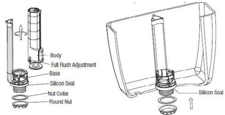
1. Rotate the Body of Flush Valve anticlockwise and take it out from Base. Unscrew Round nut and Nut collar in turn from Flush valve.
