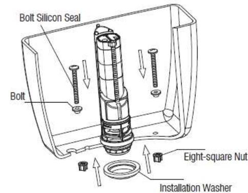
3. Take the Body of Flush valve back to Base and rotate it clockwise. Knot Installation washer to Round nut and put Tank on the right place of Bowl. Then insert Tank to Bowl bolt with Bolt silicon seal in the bolt hole (as picture) and screw Eight-square Nut to Tank to Bowl Bolt tightly. Adjust the partial flush volume by moving Partial flush cup up or down.
