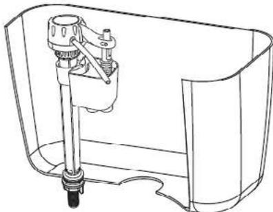
2. After connecting Water supply pipe, adjust the fill volume by rotating Rod clockwise or anticlockwise to make Small tank move up or down.
